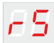
Fig. 29 Information displayed if a bay unit does have a configured network address.
