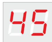
Fig. 20 Information displayed if a bay unit does have a configured network address.
